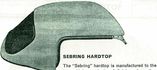
The "Sebring" hardtop is manufactured to the same high standards of finish and weather proofing and differs only in the method of fixing
