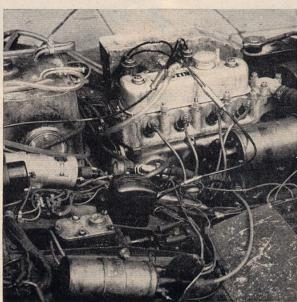
Wiring and tubing writhes around the 70 bhp Sprite engine shown here with Amal carburetors, cold air box, two coils. Note spare fuel tank.
