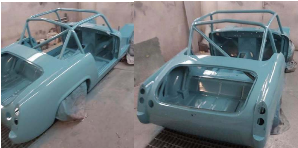
John Collinsons bespoke roll cage to fit under his Early Ashley hardtop. Note the earlier screen is slightly lower than the later one on Andrew Giles car. © John Collinson
