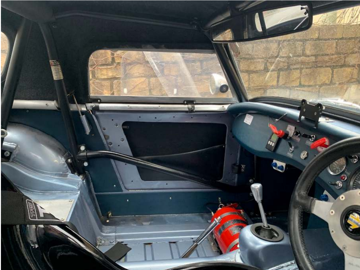
The Inside of my car showing cage, door bars, dash and full trim!! You can also see the Extinguisher and nozzles on the dash. © Mark Turner
