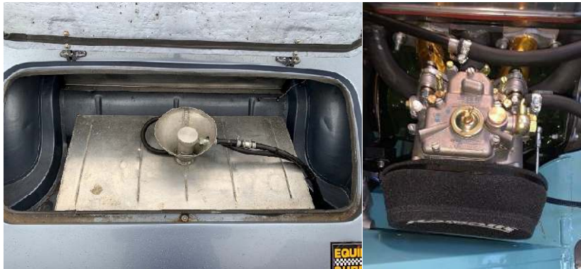
My Fuel tank Installation showing splash bowl (left) © Mark Turner and John Collinson's Weber carburettor installation showing with short trumpets and inlet manifold you can get away without inner arch modifications. (right) © John Collinson
