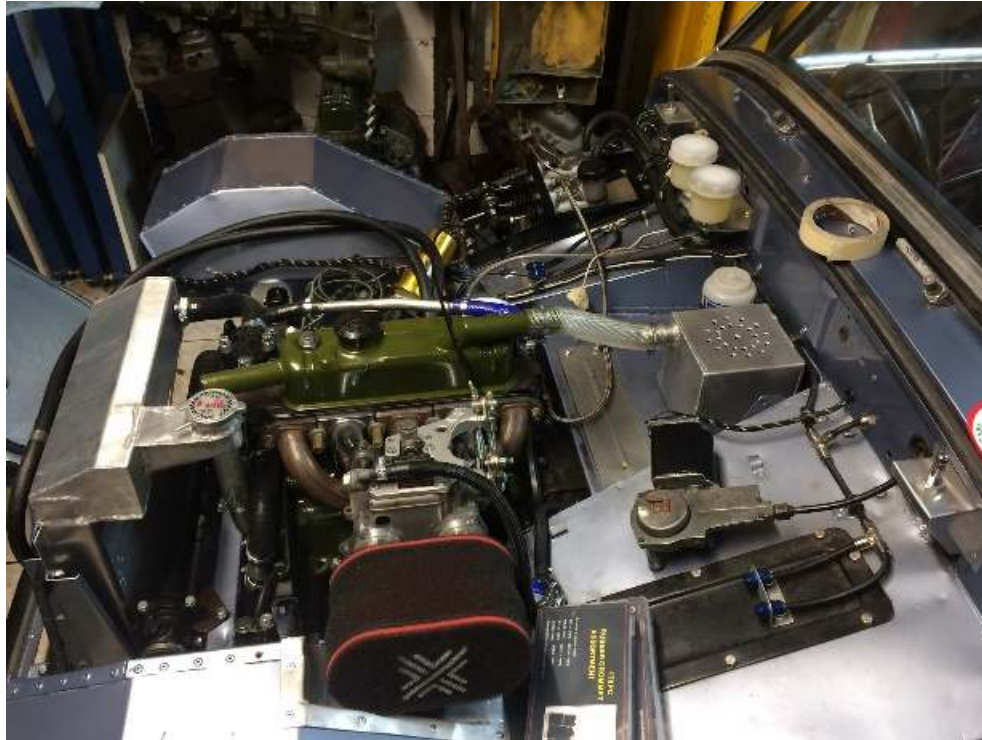
Overview of my engine bay showing the inner wing cut out, Pedal box, catch tank and extinguisher nozzles @Mark Turner
