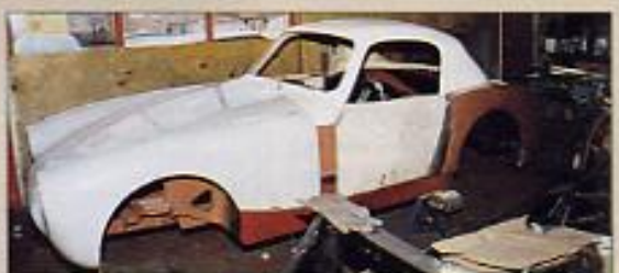
The Sebring bodywork has just been fitted. Doors, sills, rear wing and shroud are steel Froggye panels, whilst the one piece front and hardtop, with its screen, surround and scuttle, are the parts Brian Archer supplied.
