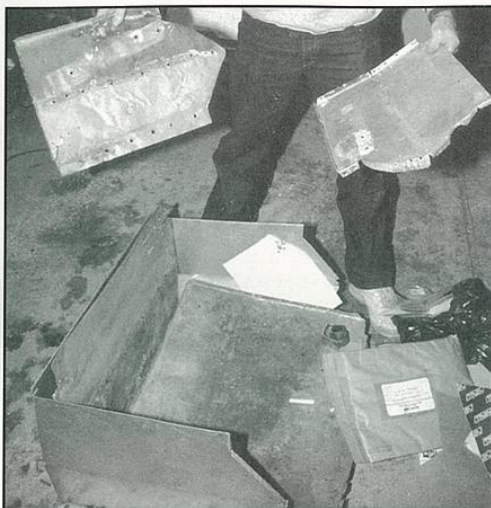
Left: Underside of the bonnet, as is. Center: Roger Sieling holds the original end panels for the boot/fuel cell structure. The original floor is in the bottom of his fabricated replacement. Right: The boot lid, like the bonnet, in its current condition. Above Roger's head is the rear shroud waiting for attention.
